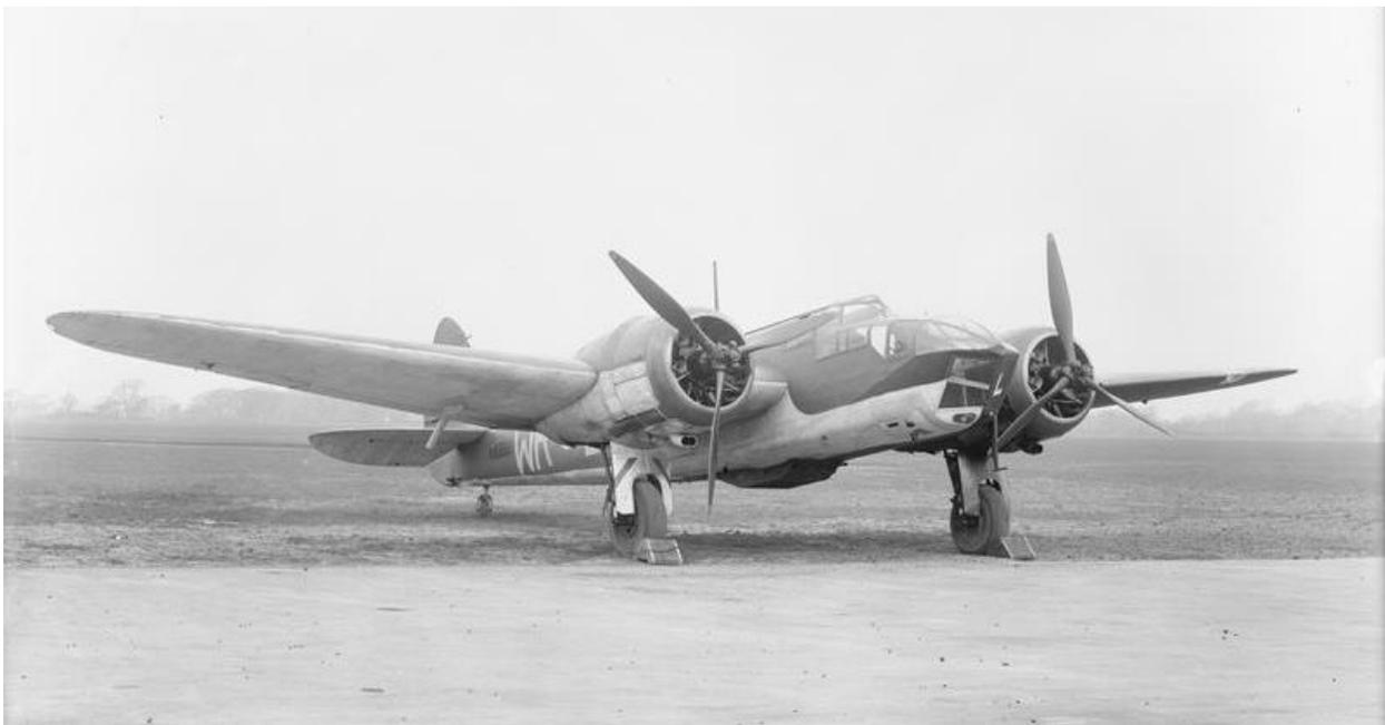
A No 248 Squadron (RAF) Bristol Blenheim Mk IVF with the characteristic extended nose and gun pack for fighter missions on its underbelly. (IWM)
